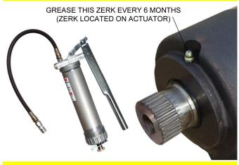
USE OF HIGH PRESSURE GREASE CAN BLOW OUT THE SEALS, LEADING TO LEAKS/SEAL DAMAGE!
