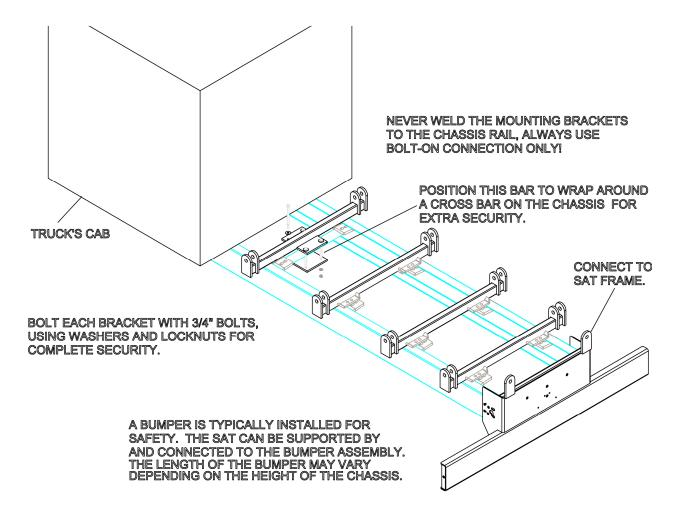
Always mount the bumper D50401hd to the end of the frame and joint it to the SAT base frame with the hardware. It supports the base frame during dumping operations.
