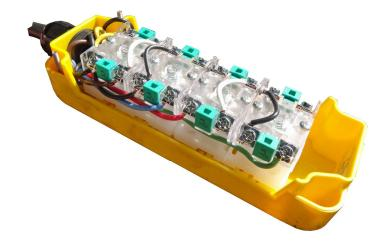
The pendant comes prewired. If repairs are necessary, re-wire the pendant as shown.
