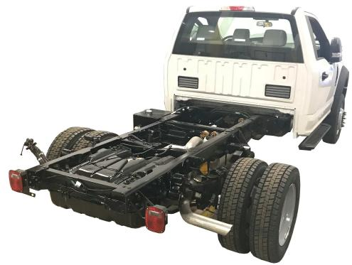
Please be sure to use a pick-up truck with a chassis capacity of 12000 lbs minimum of payload for an 8 yard, and 14600 lbs. minimum of payload for 10 yards. Please add to the payload chassis capacity weight, any other equipment planned to use. The bed floor should be approximately 33 3/4" from the ground. The brakes and suspension should be sized appropriately for these loads.
