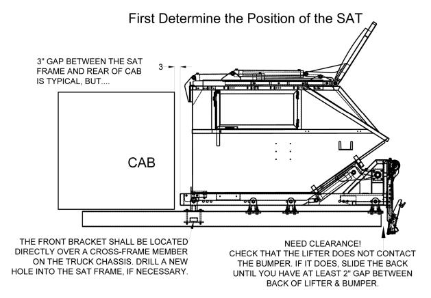
\*THE SAT FRAME IS PRE-DRILLED, BUT DUE TO VARIATIONS IN THE TRUCKS, IT MAY BE NECESSARY TO DRILL A NEW HOLE THAT BEST SUITS YOUR INSTALL.
