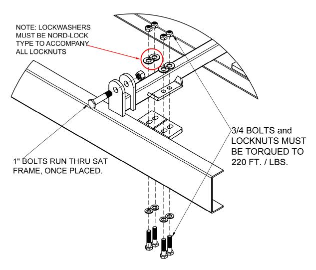
Never weld mounting brackets to the truck chassis rails. Chassis rails flex during driving, which will crack the welds. Only bolts should be used.
