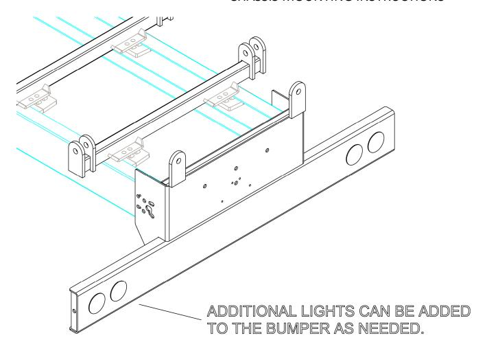
The Perkins bumper comes with x3 1" red lights in the center, and one 1" light on either end. It includes license plate mounting holes, license plate light. Extra lights can be mounted to the bumper (optionally).
